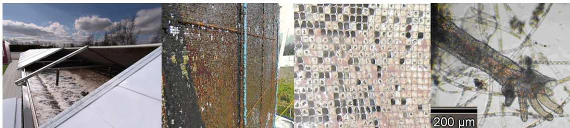
Fig. 3 – From left to right: operational worm reactor; carrier material with worm biomass; zoom in on carrier material with mesh size of 5 mm; Aulophorus furcatus under microscope.
